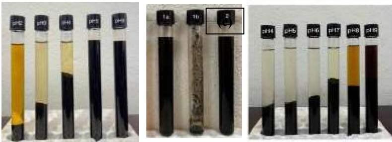
Figure 3.18. a) Effect of pH on the precipitation of HEs (Humic Extract); b) Mixture of HANPs and HEs (1), solid phase separated from HANPs/HEs after 2 days (2); c) Mixture of WSC-stabilized HANPs and HEs at a volume ratio of 3/7 at different pH levels.
